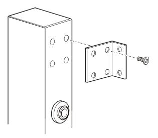
2. Install the Rack PDU on a vertical mounting rail in your rack or enclosure.
